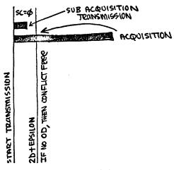
HHEN A STATION DESIRES TO TRANSMIT, IT WAITS UNTIL THE ETHER IS EMPTY AND THE SLOT COUNTER IS ZERO. IT THEN BEGINS TRANSMISSION, THE PLACING OF BITS INTO THE ETHER.
